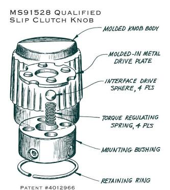
**Slip Clutch** knob design utilizes a molded-in metal drive plate in conjunction with a spring loaded sphere mechanism which provides protection against over torquing and damage of the control/component.
